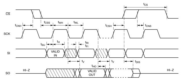
Figure 2. Synchronous Data Timing
