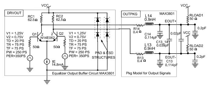
Figure 1. Equalizer output stage for the MAX3801 including a simplified package model.
