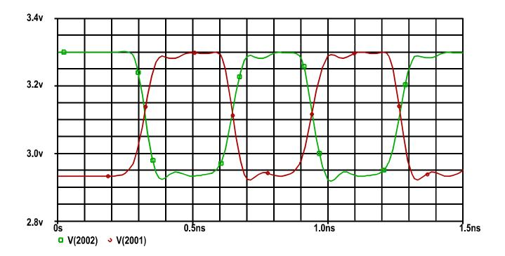
Figure 3. PSPICE simulation waveform showing the response of the output driver. Levels and rise times with the data sheet. Note as per Table 1, the waveforms are labeled V(2001), V(2002) for V(EOUT+) and V(EOUT-)
