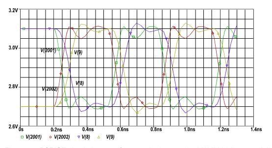
Figure 4. PSPICE simulation waveforms at the input to the MAX3801 Input model.
