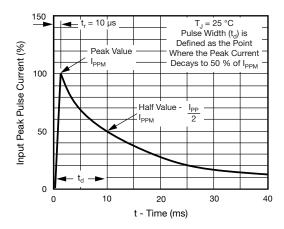
Fig. 3 - Pulse Waveform
