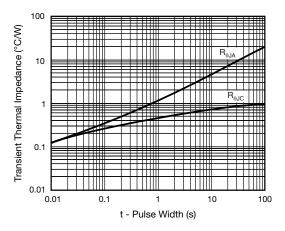
Fig. 7 - Typical Transient Thermal Impedance
