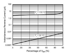
Fig. 6 - Typical Reverse Characteristics
