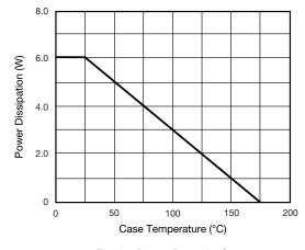
Fig. 1 - Power Derating Curve
