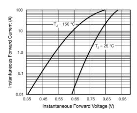
Fig. 5 - Typical Instantaneous Forward Characteristics
