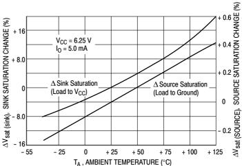
Figure 8. f<sub>out</sub>, Saturation Change versus Temperature
