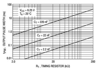
Figure 3. f<sub>out</sub>, Pulse Width versus Timing Resistor
