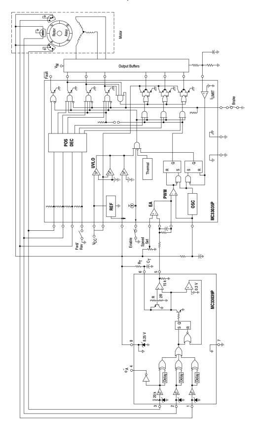
Figure 2. Typical Closed Loop Speed Control Application
