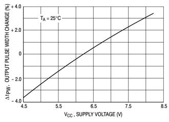
Figure 5. f<sub>out</sub>, Pulse Width Change versus Supply Voltage
