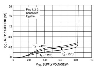
Figure 6. Supply Current versus Supply Voltage
