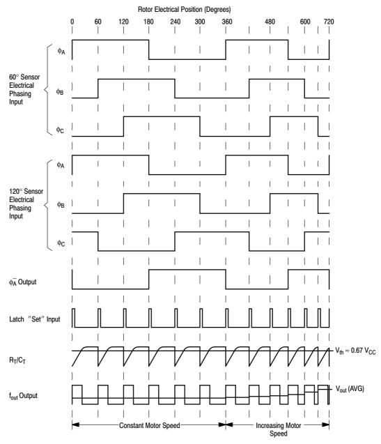
Figure 1. Typical Three Phase, Six Step Motor Application
