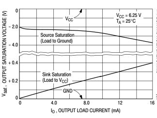
Figure 7. f<sub>out</sub>, Saturation versus Load Current
