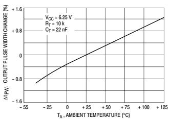
Figure 4. f<sub>out</sub>, Pulse Width Change versus Temperature
