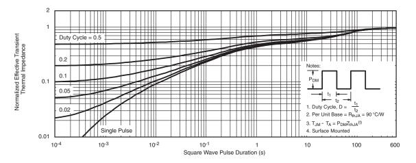
Normalized Thermal Transient Impedance, Junction-to-Ambient
