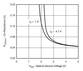
**On-Resistance vs. Gate-to-Source Voltage**
