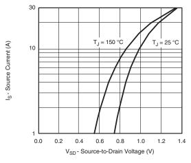
Source-Drain Diode Forward Voltage
