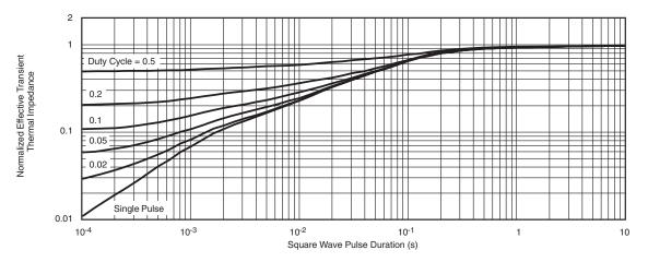
Normalized Thermal Transient Impedance, Junction-to-Foot
