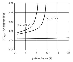
**On-Resistance vs. Drain Current**
