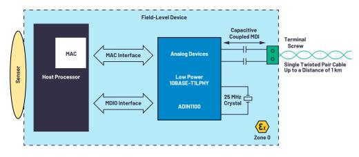
Figure 3. Field-level device connectivity with a 10BASE-T1L PHY.
