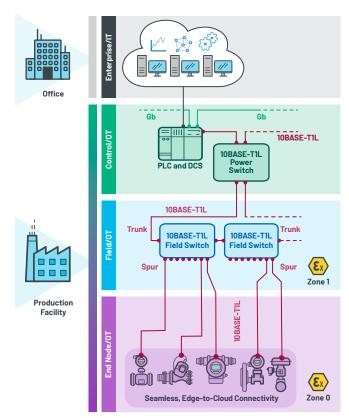
Figure 4. 10BASE-T1L network topology for the process industry.
