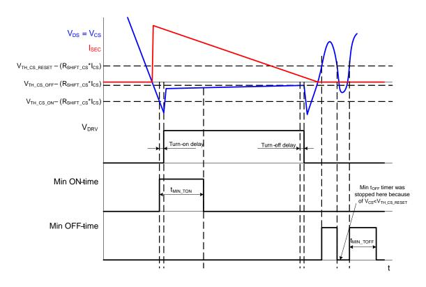
The  $t_{MIN\_TON}$  and  $t_{MIN\_TOFF}$  are adjustable by  $R_{MIN\_TON}$  and  $R_{MIN\_TOFF}$  resistors
