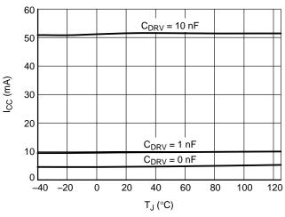
Figure 12. Current Consumption,  $V_{CC}$  = 12 V,  $V_{CS}$  = -1 to 4 V,  $f_{CS}$  = 500 kHz, ver. D
