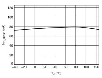
Figure 10. Current Consumption,  $V_{CC} = V_{CCOFF} - 0.1 \text{ V}$ ,  $V_{CS} = 0 \text{ V}$ , ver. D
