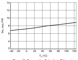
Figure 29. Propagation Delay from Trigger to **Driver Output Off**
