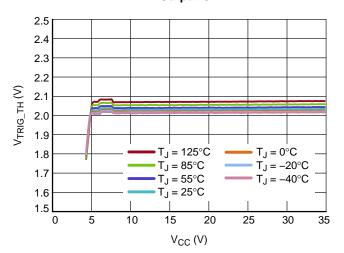
Figure 25. Trigger Threshold,  $V_{CC}$  = 12 V
