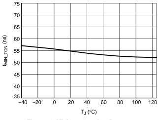
Figure 31. Minimum On–time  $R_{MIN\_TON} = 0 \Omega$
