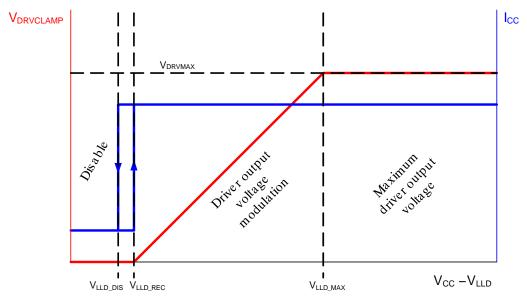
Figure 74. LLD Voltage to Driver Clamp and Current Consumption Characteristic (DRV Unloaded)
