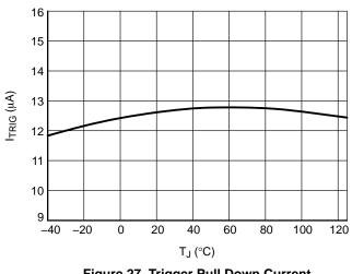
Figure 27. Trigger Pull Down Current
