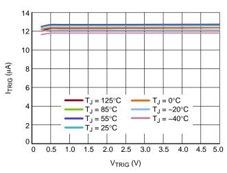
Figure 28. Trigger Pull Down Current,  $V_{CC} = 12 V$
