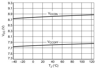
Figure 8. V<sub>CCON</sub> and V<sub>CCOFF</sub> Levels, ver. B, C
