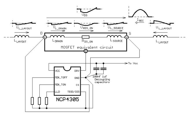
Figure 47. SR System Connection Including MOSFET and Layout Parasitic Inductances in LLC Application
