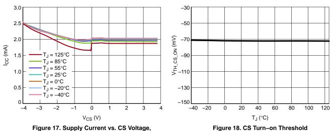
Figure 17. Supply Current vs. CS Voltage,  $V_{CC} = 12 V$
