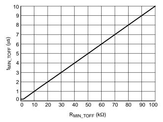
Figure 70. MIN\_TOFF Adjust Characteristics
