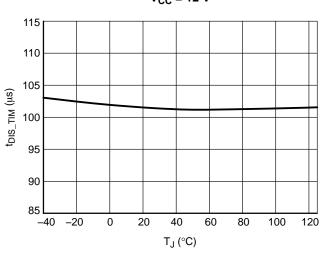
Figure 30. Delay to Disable Mode, V<sub>TRIG</sub> = 5 V
