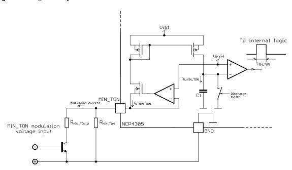
Figure 71. Possible Connection for MIN\_T<sub>ON</sub> and MIN\_T<sub>OFF</sub> Modulation
