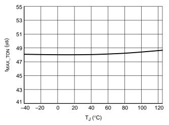
Figure 43. Maximum On–time,  $V_{MAX\_TON} = 0.3 \text{ V, ver. Q}$
