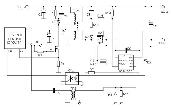
Figure 67. Primary Triggering in Deep CCM Application Using Trigger Transformer - NCP4305A, B, C or D
