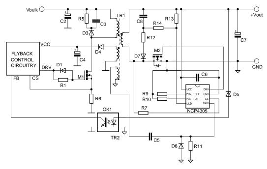
Figure 66. Primary Triggering in Deep CCM Application Using Auxiliary Winding - NCP4305A, B, C or D
