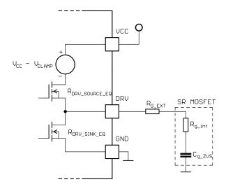
Figure 85. Equivalent Schematic of Gate Drive Circuitry
