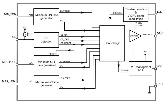
Figure 6. Internal Circuit Architecture - NCP4305Q (CCM QR) with MAX\_TON
