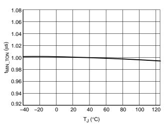
Figure 32. Minimum On–time  $R_{MIN\_TON}$  = 10  $k\Omega$
