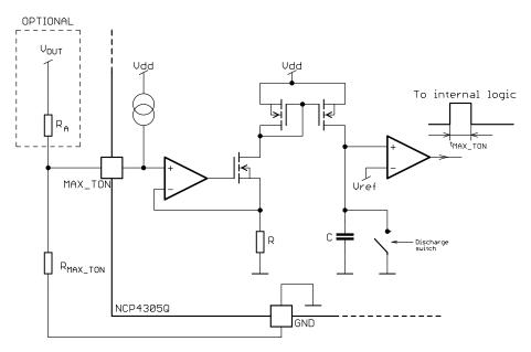
Figure 72. Internal Connection of the MAX TON Generator, NCP4305Q
