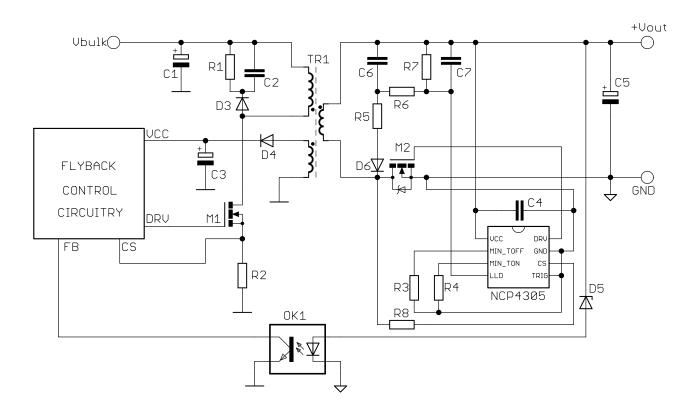
Figure 2. Typical Application Example – DCM, CCM or QR Flyback Converter with optional LLD and Disabled TRIG
