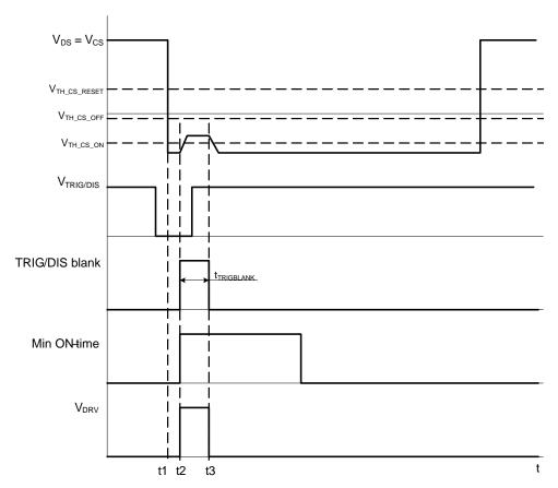
Figure 53. Trigger Input Functionality Waveforms - Trigger Blanking
