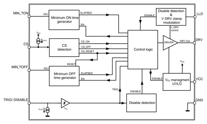
Figure 5. Internal Circuit Architecture - NCP4305A, B, C, D
