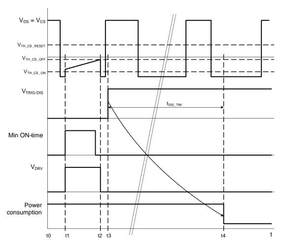
Figure 58. Trigger Input Functionality Waveforms - Disable Mode Activation
