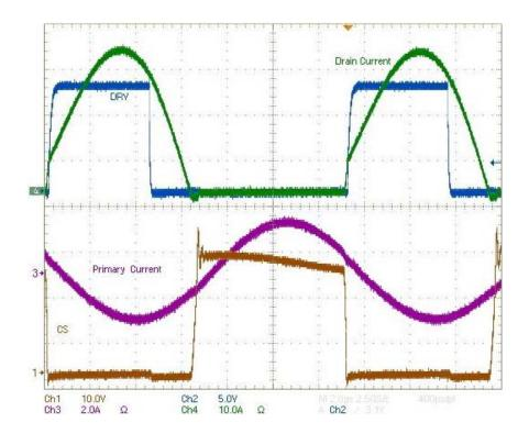
Figure 48. Waveforms From SR System Implemented in LLC Application and Using MOSFET in TO220 Package
