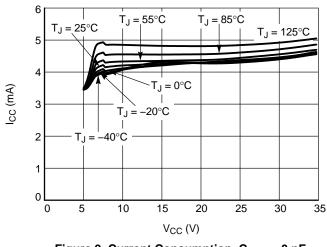
Figure 9. Current Consumption,  $C_{DRV} = 0$  nF,  $f_{CS} = 500$  kHz, ver. D
