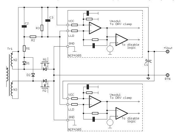
Figure 79. NCP4305 Light Load Detection in LLC Topology
