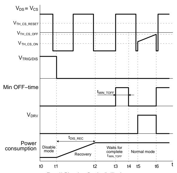
Figure 63. Trigger Input Functionality Waveforms
