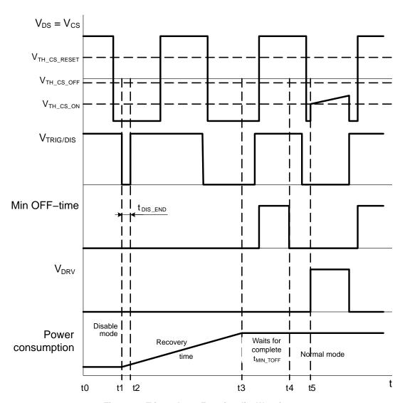
Figure 62. Trigger Input Functionality Waveforms
