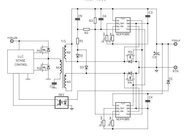
Figure 1. Typical Application Example – LLC Converter with Optional LLD and Trigger Utilization
