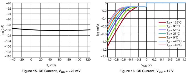
Figure 16. CS Current,  $V_{CC} = 12 \text{ V}$
