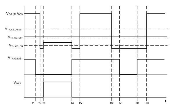
Figure 52. Trigger Input Functionality Waveforms Using the Trigger to Turn-off and Block the DRV Signal
