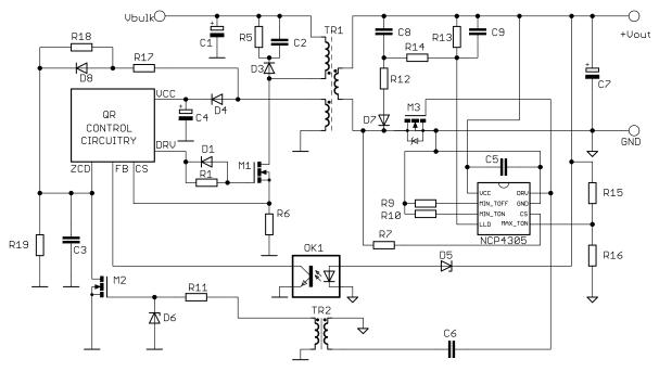
Figure 4. Typical Application Example – QR Converter – Capability to Force Primary into CCM Under Heavy Loads utilizing MAX-TON
