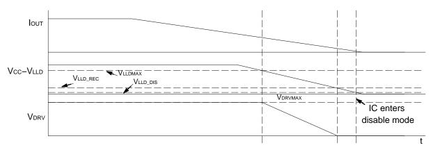
Figure 78. NCP4305 Driver Clamp Modulation Circuitry Transfer Characteristic in Flyback Application
