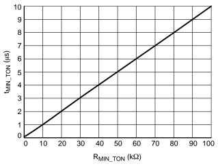
Figure 69. MIN\_TON Adjust Characteristics
