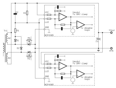
Figure 82. NCP4305 Light Load Detection in LLC Application - Other Option
