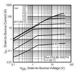
Fig. 1 - Typical Output Characteristics
