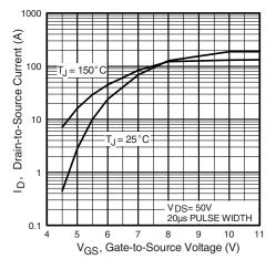
Fig. 3 - Typical Transfer Characteristics
