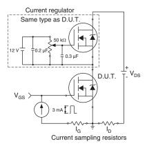
Fig. 13a - Gate Charge Test Circuit
