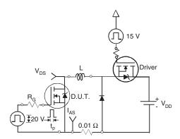
Fig. 12a - Unclamped Inductive Test Circuit
