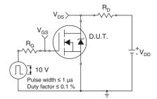
Fig. 10a - Switching Time Test Circuit
