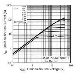
Fig. 2 - Typical Output Characteristics
