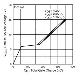
Fig. 7 - Typical Gate Charge vs. Gate-to-Source Voltage
