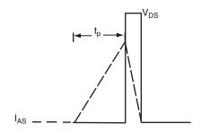
Fig. 12b - Unclamped Inductive Waveforms
