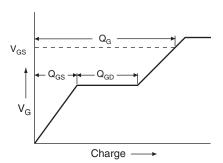
Fig. 13b - Basic Gate Charge Waveform
