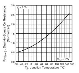
Fig. 4 - Normalized On-Resistance vs. Temperature
