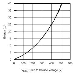
Fig. 6 - Typical Output Capacitance Stored Energy vs. V<sub>DS</sub>
