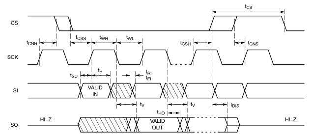
Figure 2. Synchronous Data Timing
