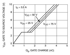
Figure 7. Gate Charge Characteristics
