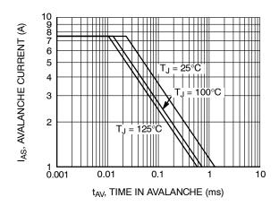
Figure 9. Unclamped Inductive Switching Capability
