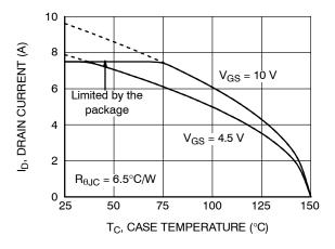
Figure 11. Maximum Continuous Drain Current vs. Case Temperature
