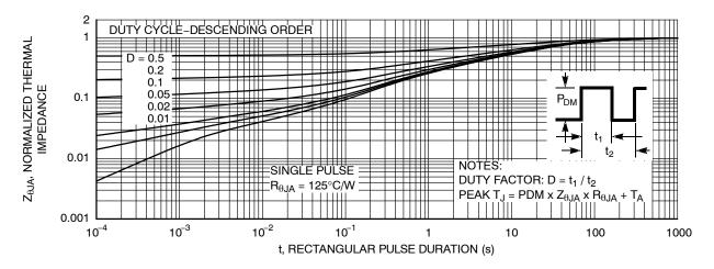
Figure 14. Junction-to-Ambient Transient Thermal Response Curve
