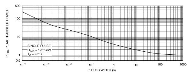
Figure 13. Single pulse Maximum Power Dissipation
