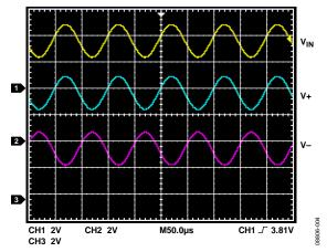
Figure 4. V<sub>IN</sub>, V+, and V- for Figure 3 Circuit at 100 kSPS Update Rate
