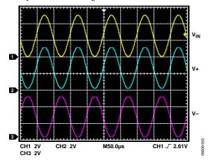
Figure 2. V<sub>IN</sub>, V+, and V- for Figure 1 Circuit at 100 kSPS Update Rate
