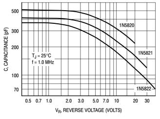
Figure 10. Typical Capacitance
