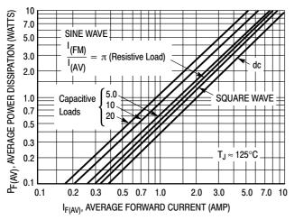
Figure 6. Forward Power Dissipation 1N5820-22
