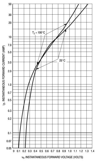
Figure 7. Typical Forward Voltage
