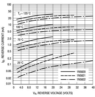
**Figure 9. Typical Reverse Current**
