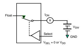
Figure 5. On Leakage
