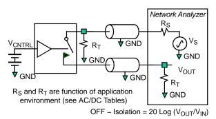
Figure 10. Channel Off Isolation
