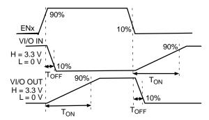
Figure 8. Turn On/Off Waveforms
