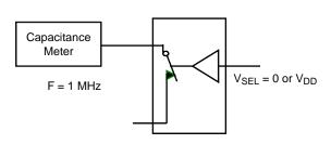
Figure 13. Channel On Capacitance
