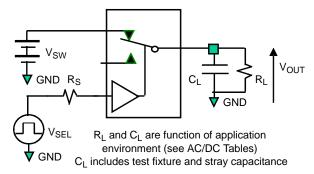
Figure 7. Test Circuit Load
