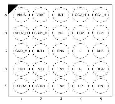
Figure 2. Pin Assignment (Top Through View)
