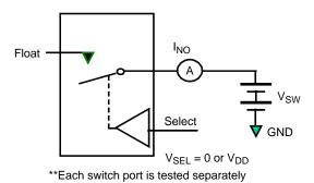
Figure 4. Off Leakage (loz)
