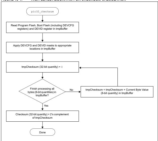
Equation 18-1 provides a formula to calculate the checksum for a PIC32 device.
