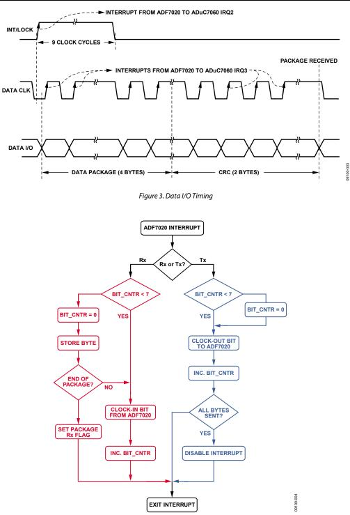
Figure 4. Interrupt Service Routines for Handling Rx and Tx Data
