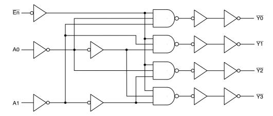
Figure 4. Expanded Logic Diagram (1/2 of Device)
