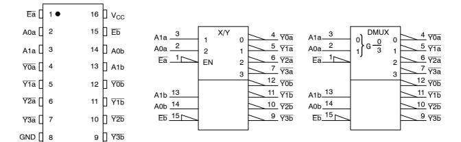
Figure 1. Pin Assignment
