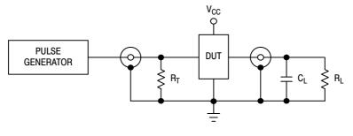
$\begin{array}{l} C_L = 50 \text{ pF or equivalent (Includes jig and probe capacitance)} \\ R_L = R_1 = 500 \ \Omega \text{ or equivalent} \\ R_T = Z_{OUT} \text{ of pulse generator (typically 50 } \Omega) \end{array}$
