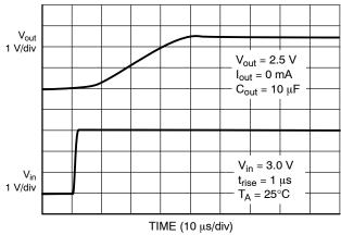
Figure 22. Startup Transient (Vout = 2.5 V)
