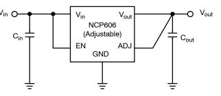
Figure 6. NCP606 Typical Application Circuit for Adjustable Version (V<sub>out</sub> = 1.25 V)
