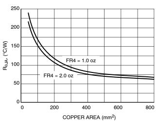
Figure 23. Thermal Resistance vs. Copper Area
