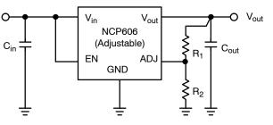
Figure 4. NCP606 Typical Application Circuit for Adjustable Version (1.25 V <  $V_{out} \le 5.0$  V)
