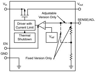
Figure 8. NCP606 Simplified Block Diagram
