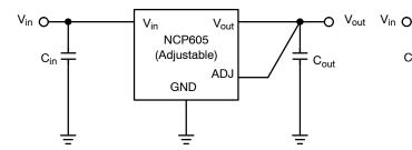
Figure 5. NCP605 Typical Application Circuit for Adjustable Version (V<sub>out</sub> = 1.25 V)
