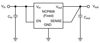
Figure 2. NCP606 Typical Application Circuit for Fixed Version (1.5 V, 1.8 V, 2.5 V, 2.8 V, 3.0 V, 3.3 V, 5.0 V)
