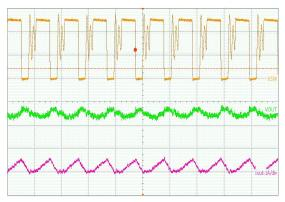
(V<sub>IN</sub> = 5 V, I<sub>LOAD</sub> = 100 mA, L = 3.3  $\mu$ H, C<sub>OUT</sub> = 2 x 22  $\mu$ F) Upper Trace: L<sub>X</sub> Pin Switching Waveform, 2 V/div Middle Trace: Output Ripple Voltage, 20 mV/div Lower Trace: Inductor Current, 1 A/div
