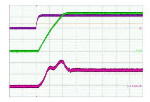
(V  $_{IN}$  = 5 V, I  $_{LOAD}$  = 100 mA, L = 3.3  $\mu H,~C_{OUT}$  = 2 x 22  $\mu F)$
