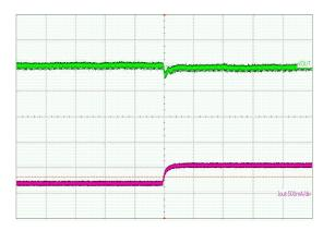
(V<sub>IN</sub> = 5 V, I<sub>LOAD</sub> = 100 mA, L = 3.3 H, C<sub>OUT</sub> = 2 x 22  $\mu$ F) Upper Trace: Output Dynamic Voltage, 100 mV/div Lower Trace: Output Current, 500 mA/div Time Scale: 200  $\mu$ s/div
