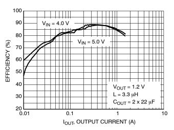
Figure 14. Efficiency vs. Output Current for  $V_{OUT}$  = 1.2 V
