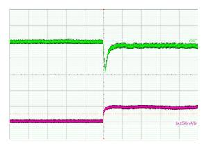
(V<sub>IN</sub> = 5 V, I<sub>LOAD</sub> = 100 mA, L = 3.3  $\mu$ H, C<sub>OUT</sub> = 2 x 22  $\mu$ F) Upper Trace: Output Dynamic Voltage, 100 mV/div Lower Trace: Output Current, 500 mA/div
