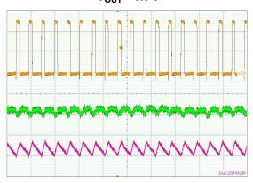
(VIN = 5 V, ILOAD = 400 mA, L = 3.3  $\mu H,~C_{OUT}$  = 2 x 22  $\mu F)$ Upper Trace: LX Pin Switching Waveform, 2 V/div Middle Trace: Output Ripple Voltage, 20 mV/div Lower Trace: Inductor Current, 1 A/div
