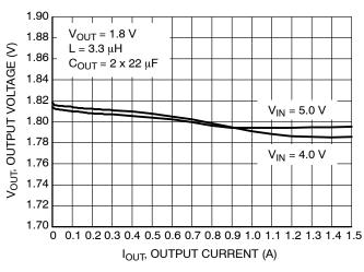
Figure 11. Load Regulation for V<sub>OUT</sub> = 1.8 V
