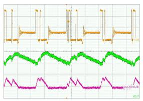
(V  $_{IN}$  = 5 V, I  $_{LOAD}$  = 100 mA, L = 3.3  $\mu H,~C_{OUT}$  = 2 x 22  $\mu F)$ Upper Trace: LX Pin Switching Waveform, 2 V/div Middle Trace: Output Ripple Voltage, 20 mV/div Lower Trace: Inductor Current, 200 mA/div
