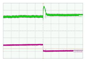
(VIN = 5 V, I<sub>LOAD</sub> = 100 mA, L = 3.3  $\mu$ H, C<sub>OUT</sub> = 2 x 22  $\mu$ F) Upper Trace: Output Dynamic Voltage, 100 mV/div Lower Trace: Output Current, 500 mA/div Time Scale: 200  $\mu$ s/div
