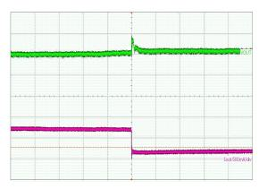
(V<sub>IN</sub> = 5 V, I<sub>LOAD</sub> = 100 mA, L = 3.3 H, C<sub>OUT</sub> = 2 x 22  $\mu$ F) Upper Trace: Output Dynamic Voltage, 100 mV/div Lower Trace: Output Current, 500 mA/div Time Scale: 200  $\mu$ s/div
