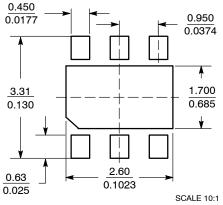
Electronic versions are uncontrolled except when accessed directly from the Document Repository. **DOCUMENT NUMBER:** 98AON19891D Printed versions are uncontrolled except when stamped "CONTROLLED COPY" in red. **DESCRIPTION:** DFN6 3\*3 MM, 0.95 PITCH, SINGLE FLAG **PAGE 1 OF 1**
