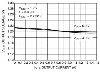
Figure 13. Load Regulation for  $V_{OUT} = 1.2 \text{ V}$
