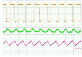
(V<sub>IN</sub> = 5 V, I<sub>LOAD</sub> = 700 mA, L = 3.3  $\mu$ H, C<sub>OUT</sub> = 2 x 22  $\mu$ F) Upper Trace: L<sub>X</sub> Pin Switching Waveform, 2 V/div Middle Trace: Output Ripple Voltage, 20 mV/div Lower Trace: Inductor Current, 1 A/div
