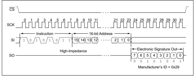
Driving  $\overline{CS}$  high after the 8-bit RDID command but before the Electronic Signature has been transmitted will still ensure the device will be taken out of Deep Power-Down mode. However, there is a delay  $T_{REL}$  that occurs before the device returns to Standby mode ( $I_{CCS}$ ), as shown in Figure 3-13.
