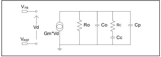
$R_C$  and  $C_C$  introduce a pole and a zero in the open loop gain.  $C_P$  does not significantly affect system stability and can be neglected.
