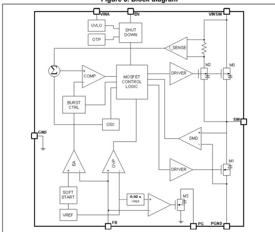
Figure 3. Block diagram
