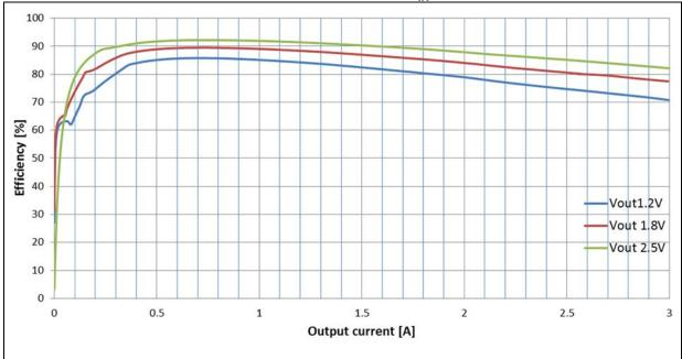
Figure 14. Efficiency curves: V<sub>IN</sub> = 4.0 V (log scale)
