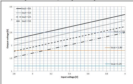
Figure 4. Maximum output voltage over loading conditions
