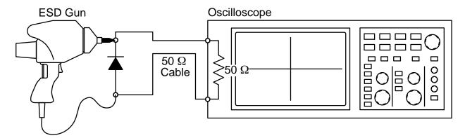
Figure 4. Diagram of ESD Test Setup
