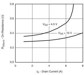
On-Resistance vs. Drain Current and Gate Voltage
