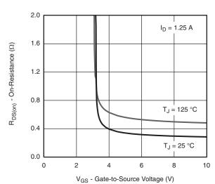
On-Resistance vs. Gate-to-Source Voltage
