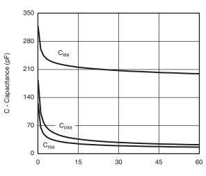
V<sub>DS</sub> - Drain-to-Source Voltage (V)
