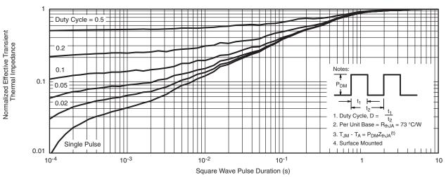
Normalized Thermal Transient Impedance, Junction-to-Foot
