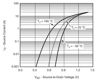
Source-Drain Diode Forward Voltage
