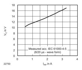
Fig. 4 - Typical Peak Clamping Voltage  $V_{\rm C}$  vs. Peak Pulse Current  $I_{\rm PP}$
