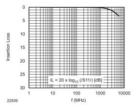
Fig. 6 - Typical Insertion Loss (IL) vs. Frequency
