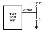
\*Includes all probe and jig capacitance
