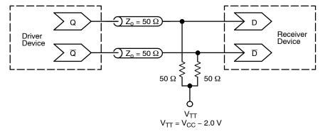
Figure 2. Typical Termination for Output Driver and Device Evaluation (See Application Note <u>AND8020/D</u> – Termination of ECL Logic Devices)
