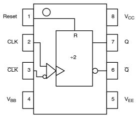
Figure 1. Logic Diagram and Pinout Assessment
