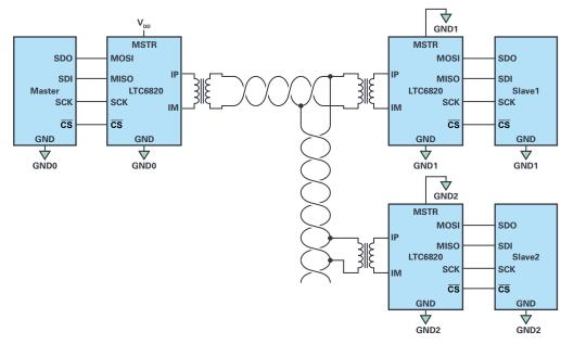
Figure 1. Isolated SPI interface for control of multiple boards (slaves) via a common master.
