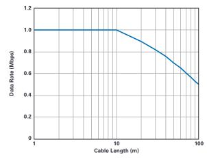
Figure 2. Data rate in relation to cable length with use of a CAT5 cable.
