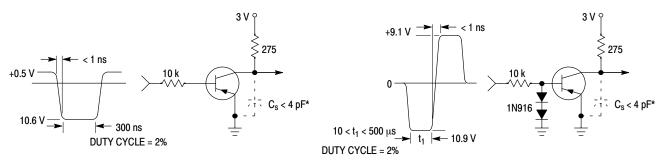
\* Total shunt capacitance of test jig and connectors
