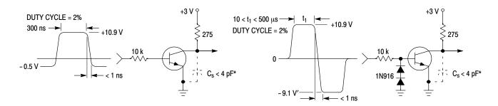
\* Total shunt capacitance of test jig and connectors
