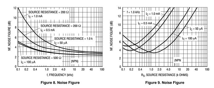
$(V_{CE} = 5.0 \text{ Vdc}, T_A = 25^{\circ}\text{C}, \text{ Bandwidth} = 1.0 \text{ Hz})$
