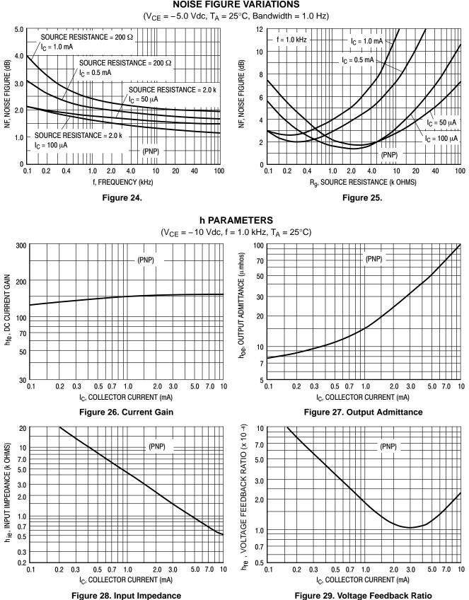
TYPICAL AUDIO SMALL-SIGNAL CHARACTERISTICS NOISE FIGURE VARIATIONS
