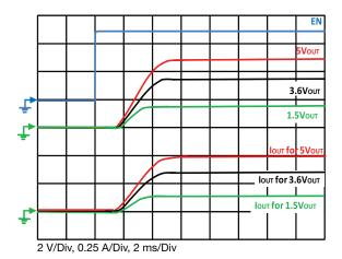
Fig. 21 - Typical Turn-On Delay, Rise Time C  $_{OUT}$  = 0.1  $\mu\text{F},$  C  $_{IN}$  = 4.7  $\mu\text{F},$  R  $_{OUT}$  = 10  $\Omega$
