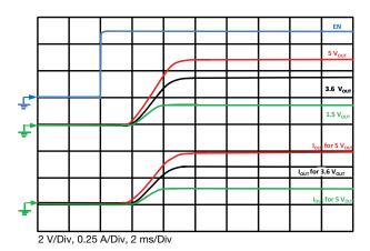
Fig. 23 - Typical Turn-On Delay, Rise Time  $C_{OUT}$  = 200  $\mu$ F,  $C_{IN}$  = 4.7  $\mu$ F,  $R_{OUT}$  = 10  $\Omega$
