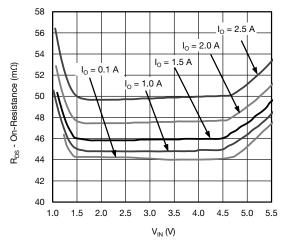
Fig. 9 -  $R_{DS(on)}$  vs.  $V_{IN}$
