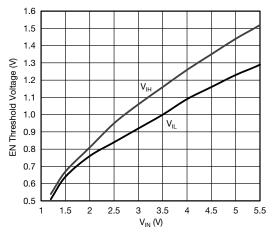
Fig. 18 - EN Threshold Voltage vs. Input Voltage
