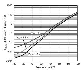
Fig. 11 - Off Switch Current vs. Temperature
