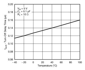
Fig. 17 - Turn-Off Delay Time vs. Temperature
