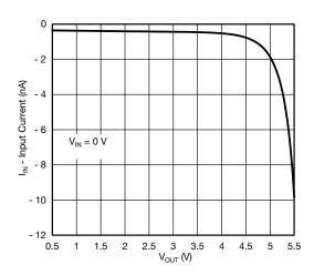
Fig. 14 - Reverse Blocking Current vs. Output Voltage
