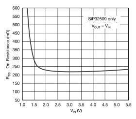
Fig. 10 - Output Pulldown vs. V<sub>IN</sub>
