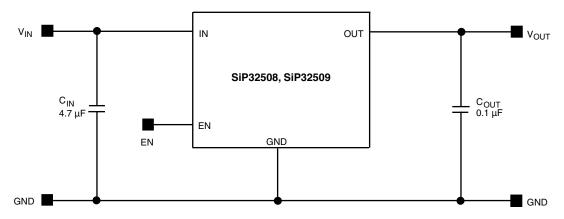
Fig. 1 - SiP32508, SiP32509 Typical Application Circuit
