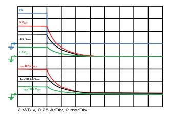
Fig. 26 - Typical Fall Time Cout = 200  $\mu$ F, C<sub>IN</sub> = 4.7  $\mu$ F, R<sub>OUT</sub> = 10  $\Omega$
