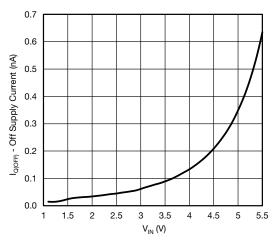
Fig. 5 - Off Supply Current vs. Input Voltage
