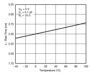
Fig. 15 - Rise Time vs. Temperature
