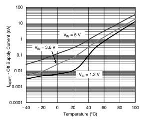
Fig. 7 - Off Supply Current vs. Temperature
