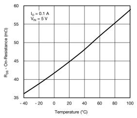
Fig. 12 - R<sub>DS(on)</sub> vs. Temperature
