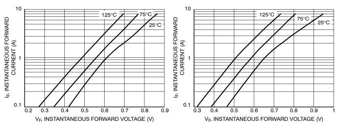
Figure 1. Typical Forward Voltage
