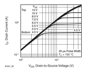
Fig. 2 - Typical Output Characteristics,  $T_C$  = 150  $^\circ C$
