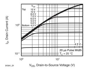
Fig. 1 - Typical Output Characteristics,  $T_C = 25 \ ^{\circ}C$
