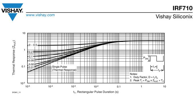
Fig. 11 - Maximum Effective Transient Thermal Impedance, Junction-to-Case
