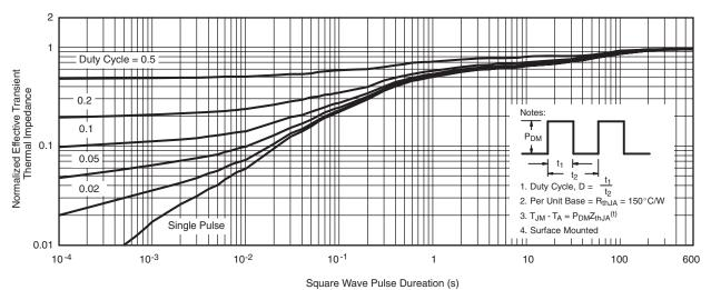
Normalized Thermal Transient Impedance, Junction-to-Ambient
