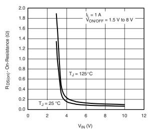
On-Resistance vs. Input Voltage
