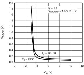
$V_{DROP}$  vs.  $V_{IN}$  at = 1 A
