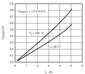
$V_{DROP}$  vs.  $I_L$  at  $V_{IN} = 5$  V
