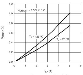
$V_{DROP}$  vs.  $I_L$  at  $V_{IN}$  = 4.5 V
