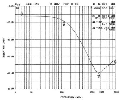
Figure 2. Insertion Loss vs. Frequency (A2-C2 to GND B1)
