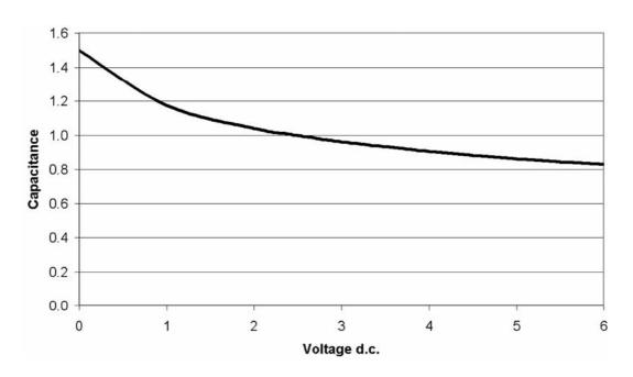
Figure 9. Filter Capacitance vs. Input Voltage over Temperature (normalized to capacitance at 2.5 VDC and 25°C)
