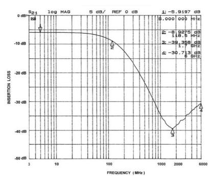
Figure 7. Insertion Loss vs. Frequency (A7–C7 to GND B4, CM1422 Only)
