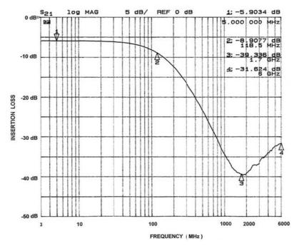
Figure 8. Insertion Loss vs. Frequency (A8–C8 to GND B4, CM1422 Only)
