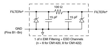
\*See Package/Pinout Diagrams for expanded pin information.
