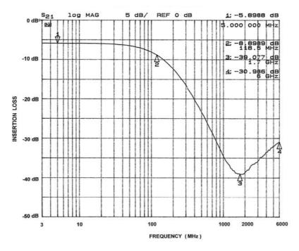
Figure 3. Insertion Loss vs. Frequency (A3-C3 to GND B2)
