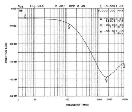
Figure 5. Insertion Loss vs. Frequency (A5-C5 to GND B3)
