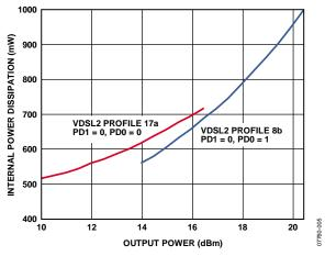
Figure 11. Internal Power Dissipation vs. Output Power
