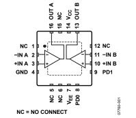
Figure 1. Thermally Enhanced, 4 mm × 4 mm, 16-Lead LFCSP\_WQ
