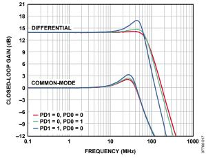
Figure 5. Small Signal Differential and Common-Mode Frequency Response; A<sub>V DIFF</sub> = 5 (See the Application Circuit in Figure 8)
