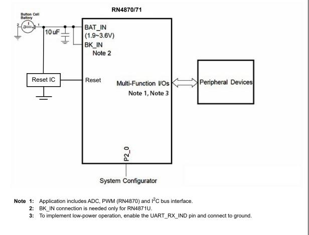
The Configuration pins on the RN4870 can also be configured through a Windows<sup>®</sup> based User Interface (UI) configuration tool, BLEDK3.
