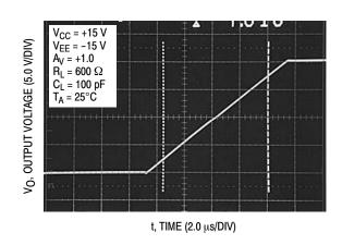
Figure 31. Non-inverting Amplifier Slew Rate
