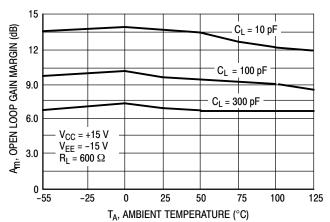
Figure 21. Open Loop Gain Margin versus Temperature
