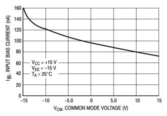
Figure 4. Input Bias Current versus Common Mode Voltage
