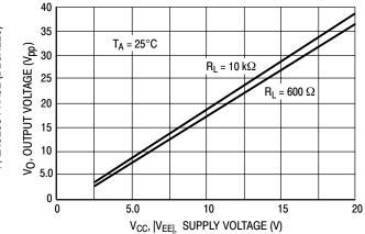
Figure 9. Output Voltage Swing versus Supply Voltage
