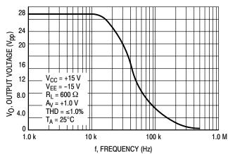
Figure 11. Output Voltage versus Frequency
