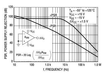
Figure 13. Power Supply Rejection versus Frequency Over Temperature
