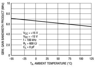
Figure 18. Gain Bandwidth Product versus Temperature
