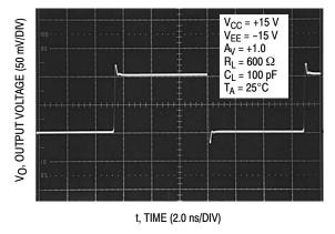
Figure 32. Small Signal Transient Response
