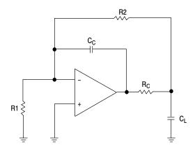
Figure 37. Compensation Circuit for High Capacitive Loads
