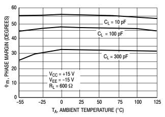
Figure 22. Phase Margin versus Temperature
