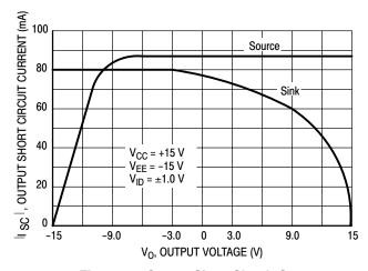
Figure 14. Output Short Circuit Current versus Output Voltage
