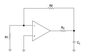
Figure 36. Compensation Circuit for Moderate Capacitive Loads
