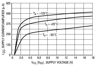
Figure 16. Supply Current versus Supply Voltage with No Load
