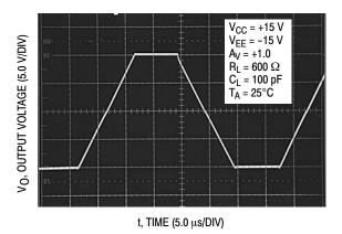
Figure 33. Large Signal Transient Response
