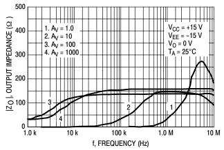
Figure 27. Output Impedance versus Frequency
