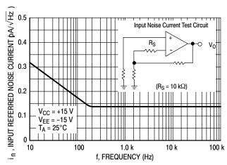
Figure 29. Input Referred Noise Current versus Frequency
