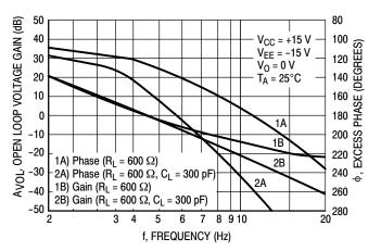
Figure 8. Voltage Gain and Phase versus Frequency
