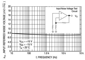
Figure 28. Input Referred Noise Voltage versus Frequency
