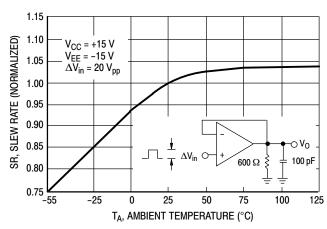
Figure 17. Normalized Slew Rate versus Temperature
