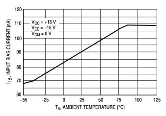
Figure 5. Input Bias Current versus Temperature
