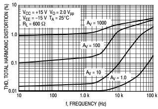
Figure 26. Total Harmonic Distortion versus Frequency
