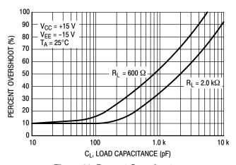
Figure 30. Percent Overshoot versus Load Capacitance
