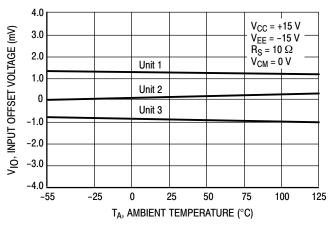
Figure 3. Input Offset Voltage versus Temperature for 3 Typical Units
