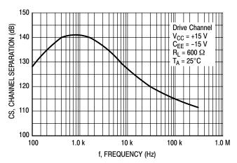
Figure 25. Channel Separation versus Frequency
