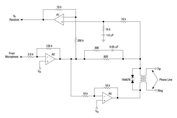
Figure 34. Telephone Line Interface Circuit
