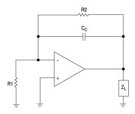
Figure 35. Compensation for High Source Impedance
