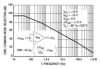
Figure 12. Common Mode Rejection versus Frequency Over Temperature
