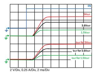
Fig. 22 - Typical Turn-on Delay, Rise Time Cout = 0.1  $\mu$ F, C<sub>IN</sub> = 4.7  $\mu$ F, R<sub>OUT</sub> = 10  $\Omega$
