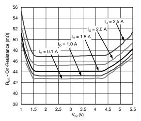
Fig. 12 - R<sub>DS(on)</sub> vs. V<sub>IN</sub>
