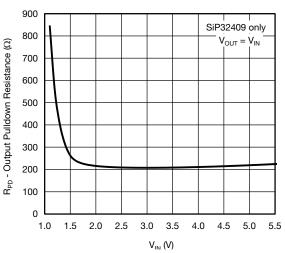
Fig. 13 - Output Pull-down Resistance vs. Input Voltage
