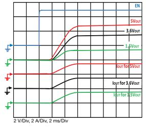
Fig. 23 - Typical Turn-on Delay, Rise Time  $C_{OUT}=200~\mu\text{F},~C_{IN}=4.7~\mu\text{F},~I_{OUT}=1.5~\text{A}$
