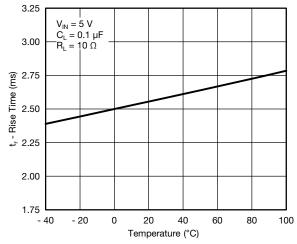
Fig. 17 - Rise Time vs. Temperature
