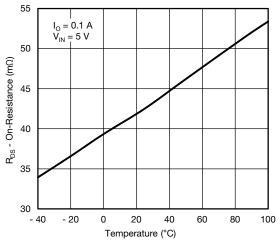
Fig. 14 - R<sub>DS(on)</sub> vs. Temperature
