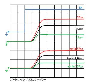
Fig. 27 - Typical Turn-on Delay, Rise Time  $C_{OUT}$  = 200  $\mu$ F,  $C_{IN}$  = 4.7  $\mu$ F,  $R_{OUT}$  = 10  $\Omega$
