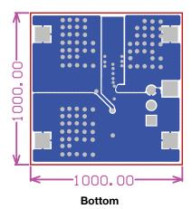
Fig. 29 - Evaluation board Layout for TDFN4 1.2 mm x 1.6 mm (type: FR4, size: 1" x 1", thickness: 0.062", copper thickness: 2 oz.)
