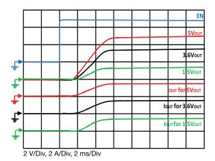
Fig. 21 - Typical Turn-on Delay, Rise Time  $C_{OUT}$  = 0.1  $\mu F,\,C_{IN}$  = 4.7  $\mu F,\,I_{OUT}$  = 1.5 A
