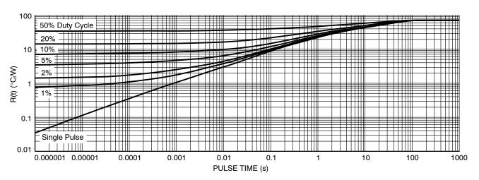
Figure 11. Thermal Response, Junction-to-Ambient
