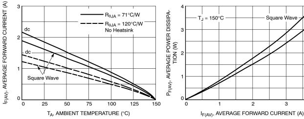
Figure 7. Current Derating, Ambient
