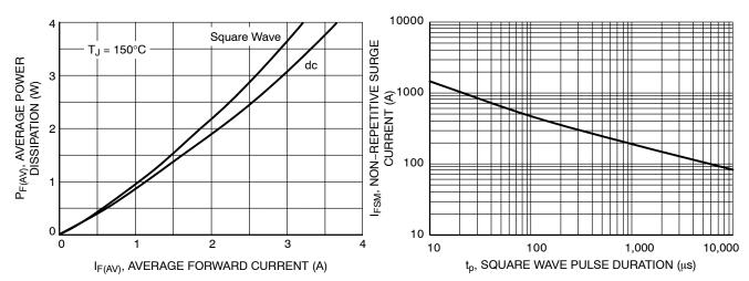
Figure 9. Maximum Forward Power Dissipation
