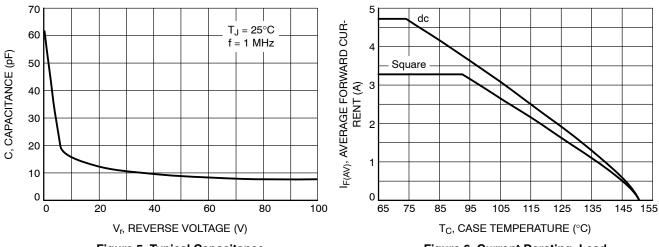
Figure 5. Typical Capacitance
