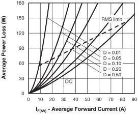
Fig. 6 - Forward Power Loss Characteristics
