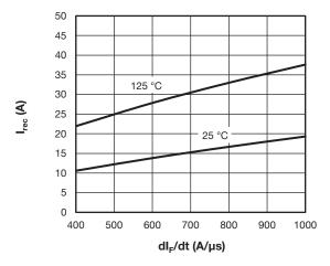
Fig. 9 - Typical Reverse Recovery vs. dl<sub>F</sub>/dt
