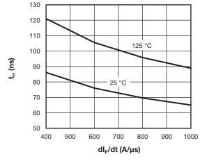
Fig. 7 - Typical Reverse Recovery Time vs. dI<sub>F</sub>/dt
