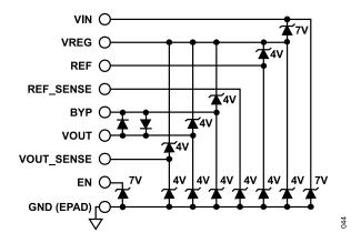
Figure 41. Simplified ESD Protection Block Diagram
