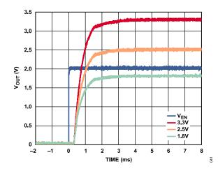
Figure 38.  $V_{OUT}$  Start-Up Time After  $V_{EN}$  Rising, at Various Output Voltages,  $V_{IN} = 5$  V,  $C_{BYP} = 1 \mu F$
