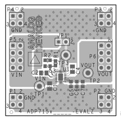
Figure 61. Sample 10-Lead LFCSP PCB Layout
