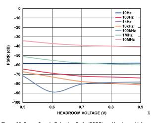
Figure 25. Power Supply Rejection Ratio (PSRR) vs. Headroom Voltage at Various Frequencies, V<sub>OUT</sub> = 1.8 V, 1.2 A Load
