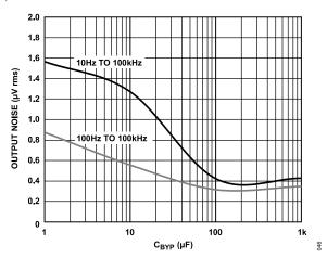
Figure 43. RMS Output Noise vs. Bypass Capacitance (CBYP)
