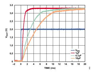
Figure 39.  $V_{OUT}$  Start-Up Time Behavior at Various Values of  $C_{BYP}$ ,  $V_{OUT}$  = 3.3
