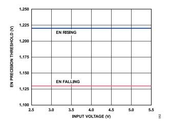
Figure 49. Typical EN Precision Threshold vs. Input Voltage (V<sub>IN</sub>)
