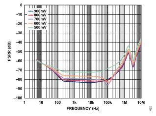
Figure 21. Power Supply Rejection Ratio (PSRR) vs. Frequency at Various Headroom Voltages, V<sub>OUT</sub> = 3.3 V, 1.2 A Load
