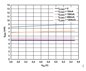
Figure 10. Ground Current ( $I_{GND}$ ) vs. Input Voltage ( $V_{IN}$ ) at Various Loads,  $V_{OUT} = 3.3 \text{ V}$
