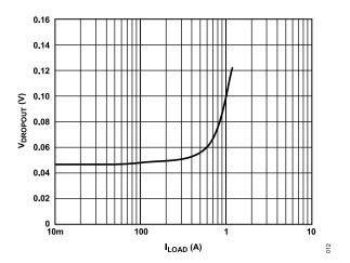
Figure 11. Dropout Voltage ( $V_{DROPOUT}$ ) vs. Load Current ( $I_{LOAD}$ ),  $V_{OUT}$  = 3.3 V
