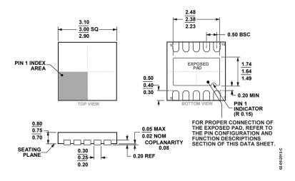
Figure 63. 10-Lead Lead Frame Chip Scale Package [LFCSP] 3 mm × 3 mm Body and 0.75 mm Package Height (CP-10-9) Dimensions shown in millimeters
