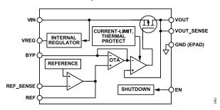
Figure 40. Simplified Internal Block Diagram
