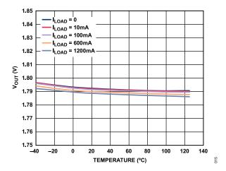
Figure 14. Output Voltage ( $V_{OUT}$ ) vs. Temperature at Various Loads,  $V_{OUT}$  = 1.8 V
