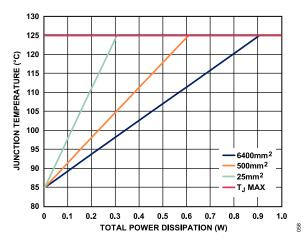
Figure 55. Junction Temperature vs. Total Power Dissipation for the 10-Lead LFCSP,  $T_A$  = 85°C
