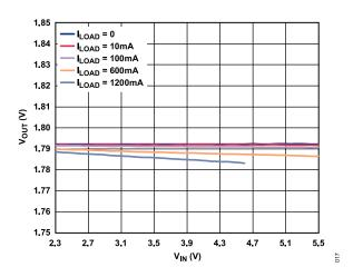
Figure 16. Output Voltage ( $V_{OUT}$ ) vs. Input Voltage ( $V_{IN}$ ) at Various Loads,  $V_{OUT} = 1.8 \text{ V}$
