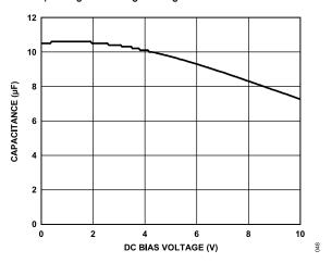
Figure 45. Capacitance vs. DC Bias Voltage
