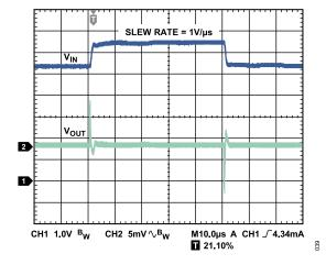
Figure 36. Line Transient Response, 1 V Input Step,  $I_{LOAD}$  = 1.2 A,  $V_{OUT}$  = 3.3 V,  $V_{IN}$  = 3.8 V, Channel 1 =  $V_{IN}$ , Channel 2 =  $V_{OUT}$
