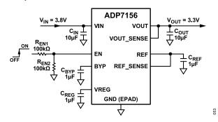
Figure 50. Typical EN Pin Voltage Divider
