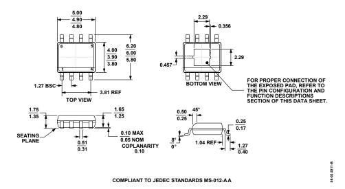
Figure 64. 8-Lead Standard Small Outline Package, with Exposed Pad [SOIC\_N\_EP]
