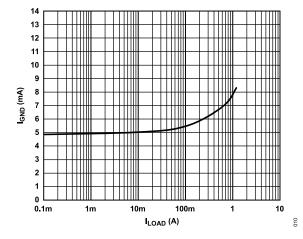
Figure 9. Ground Current ( $I_{GND}$ ) vs. Load Current ( $I_{LOAD}$ ),  $V_{OUT}$  = 3.3 V
