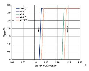
Figure 47. Typical V<sub>OUT</sub> Response to EN Pin Operation
