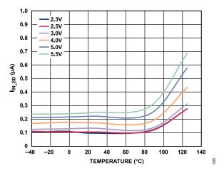
Figure 4. Shutdown Current ( $I_{\rm IN}$  <sub>SD</sub>) vs. Temperature at Various Input Voltages ( $\bar{V}_{\rm IN}$ ),  $V_{\rm OUT}$  = 1.8 V
