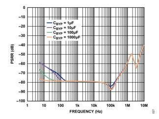
Figure 26. Power Supply Rejection Ratio (PSRR) vs. Frequency at Various  $C_{BYP}$  Values,  $V_{OUT}$  = 3.3 V,  $V_{IN}$  = 4.0 V, 1.2 A Load
