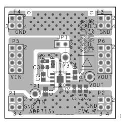
Figure 62. Sample 8-Lead SOIC PCB Layout
