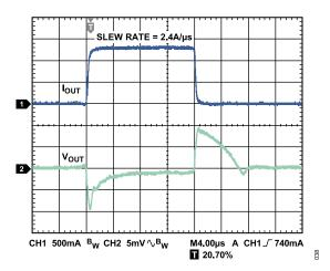
Figure 35. Load Transient Response,  $I_{LOAD}$  = 100 mA to 1.2 A,  $V_{OUT}$  = 1.8 V,  $V_{IN}$  = 2.5 V,  $C_{OUT}$  = 22  $\mu$ F, Channel 1 =  $I_{OUT}$ , Channel 2 =  $V_{OUT}$
