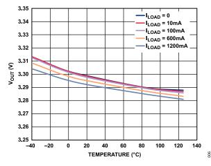
Figure 5. Output Voltage ( $V_{OUT}$ ) vs. Temperature at Various Loads,  $V_{OUT}$  = 3.3
