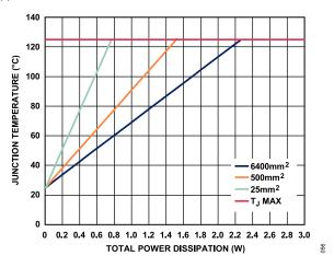
Figure 53. Junction Temperature vs. Total Power Dissipation for the 10-Lead LFCSP,  $T_{\Delta}$  = 25°C
