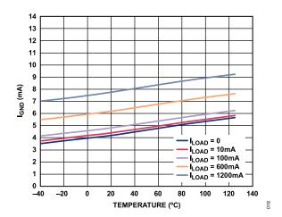
Figure 17. Ground Current ( $I_{GND}$ ) vs. Temperature at Various Loads,  $V_{OUT}$  = 1.8 V
