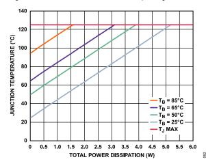
Figure 59. Junction Temperature vs. Total Power Dissipation for the 10-Lead LFCSP
