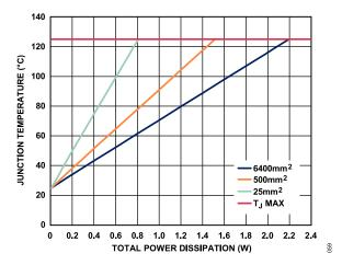
Figure 56. Junction Temperature vs. Total Power Dissipation for the 8-Lead SOIC,  $T_A$  = 25°C
