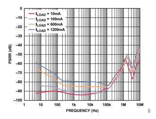
Figure 20. Power Supply Rejection Ratio (PSRR) vs. Frequency at Various Loads,  $V_{OUT} = 3.3 \text{ V}$ ,  $V_{IN} = 4.0 \text{ V}$
