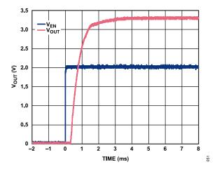
Figure 48. Typical  $V_{OUT}$  Response to EN Pin Operation ( $V_{EN}$ ),  $V_{OUT}$  = 3.3 V,  $V_{IN}$ = 5 V,  $C_{RYP}$  = 1  $\mu$ F
