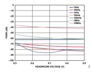
Figure 22. Power Supply Rejection Ratio (PSRR) vs. Headroom Voltage at Various Frequencies,  $V_{OUT}$  = 3.3 V, 1.2 A Load
