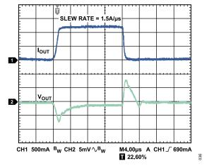
Figure 33. Load Transient Response,  $I_{LOAD}$  = 100 mA to 1.2 A,  $V_{OUT}$  = 3.3 V,  $V_{IN}$  = 4.0 V,  $C_{OUT}$  = 22  $\mu$ F, Channel 1 =  $I_{OUT}$ , Channel 2 =  $V_{OUT}$
