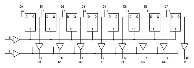
Figure 7. Expanded Logic Diagram
