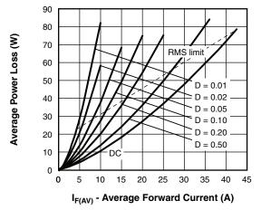
Fig. 6 - Forward Power Loss Characteristics
