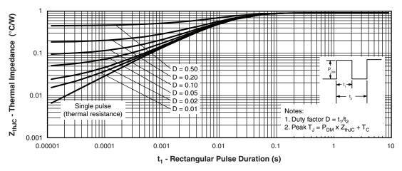
Fig. 4 - Maximum Thermal Impedance Z<sub>thJC</sub> Characteristics
