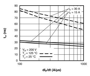
Fig. 7 - Typical Reverse Recovery Time vs. dl<sub>F</sub>/dt
