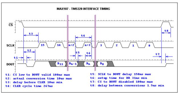
Figure 2. MAX187-TMS320 timing.
