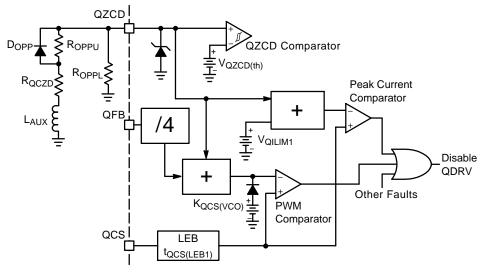
Figure 24. Overpower Compensation Circuit Schematic
