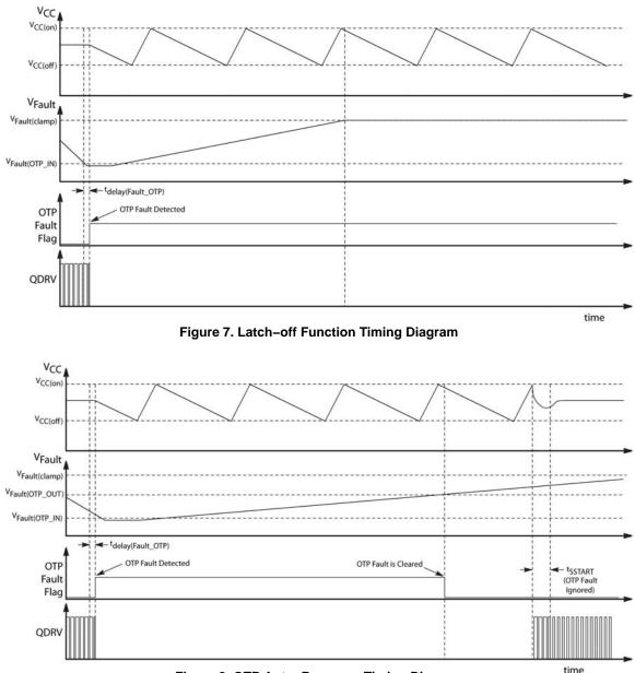
Figure 8. OTP Auto–Recovery Timing Diagram
