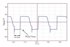
Figure 25. Auxiliary Winding Voltage Waveform
