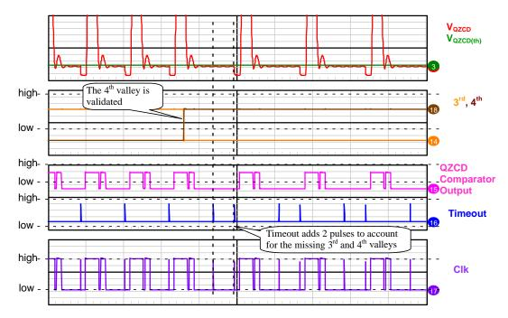
Figure 20. Timeout Operation With Missing 3<sup>rd</sup> and 4<sup>th</sup> Valleys
