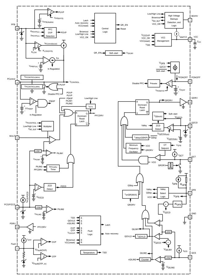
Figure 2. NCL30030 Functional Block Diagram
