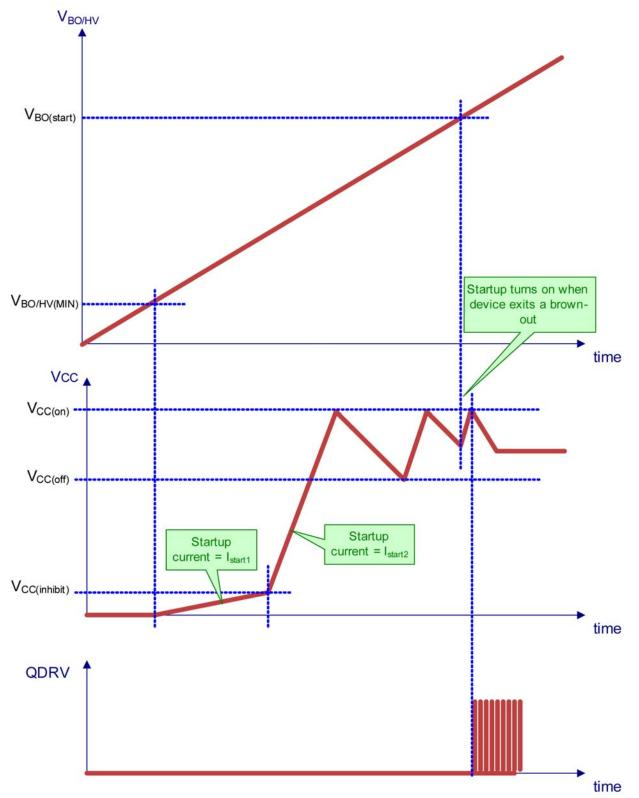
Figure 4. Startup Timing Diagram
