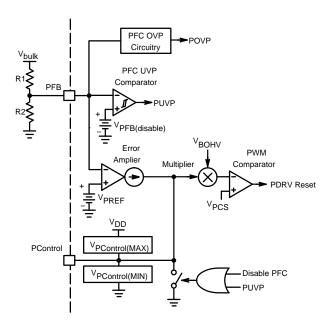
Figure 28. PFC Regulation Circuit Schematic
