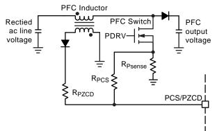
Figure 31. ZCD Winding Implementation
