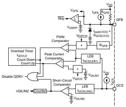
Figure 21. Current Sensing Circuitry Schematic
