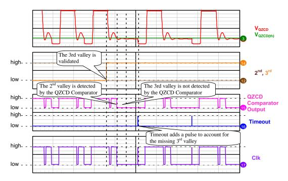
Figure 19. Timeout Operation With a Missing 3<sup>rd</sup> Valley
