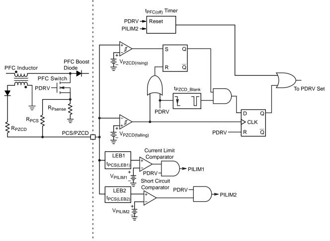
Figure 30. PFC Current Sense and ZCD Detectors Schematic
