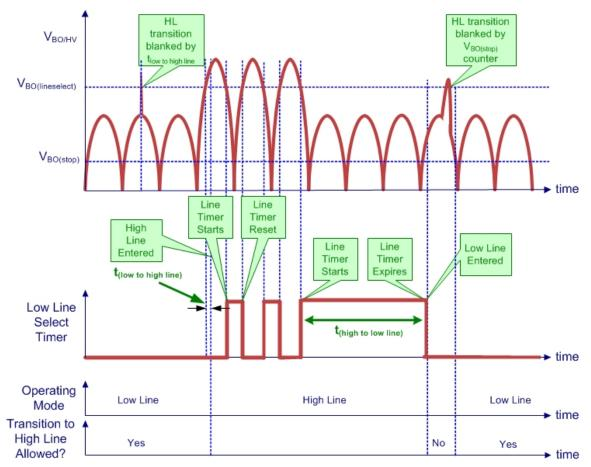
Figure 5. Line Detector Waveforms
