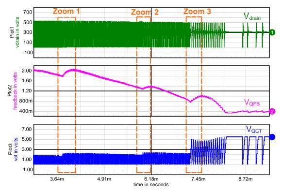
Figure 13. Operating Mode Transitions Between 2<sup>nd</sup> to 3<sup>rd</sup>, 3<sup>rd</sup> to 4<sup>th</sup> and 4<sup>th</sup> Valley to VCO Mode
