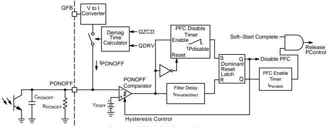
Figure 33. PFC On/Off Control Circuitry
