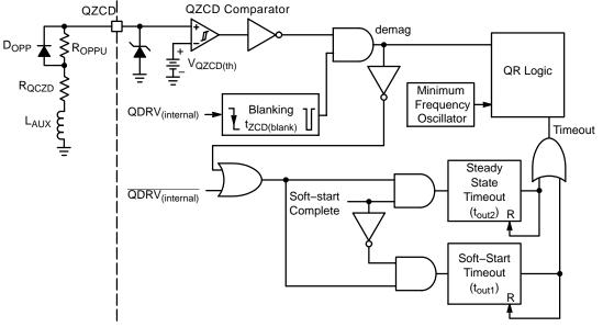
Figure 18. Timeout Period Generator Circuit Schematic
