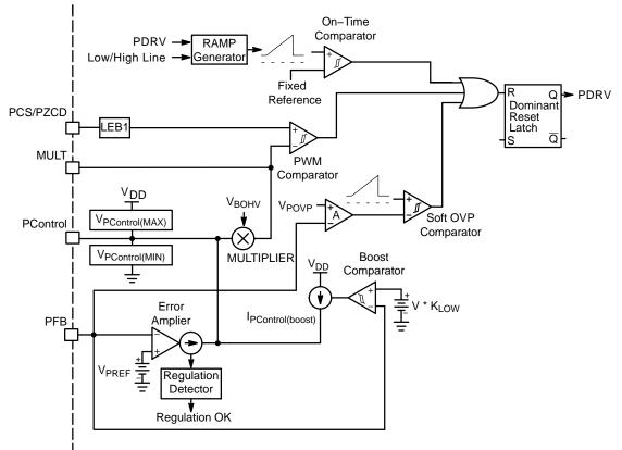
Figure 29. Boost and Soft–OVP Circuit Schematics
