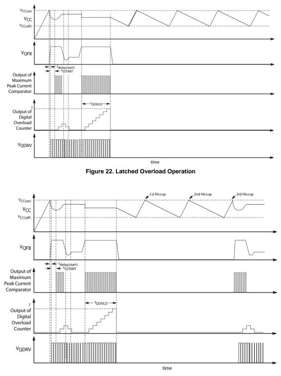
Figure 23. Auto-Recovery Overload Operation
