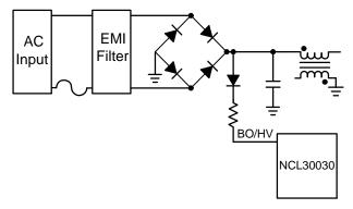
Figure 3. Brown-out and Line Voltage Detectors Configuration
