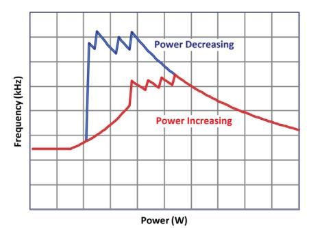
Figure 9. Valley Lockout Frequency vs Output Power Relationship
