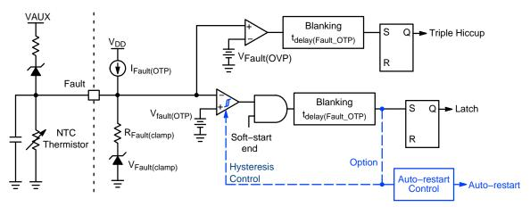
Figure 6. Fault Detection Schematic
