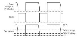
Figure 32. ZCD Winding Waveforms
