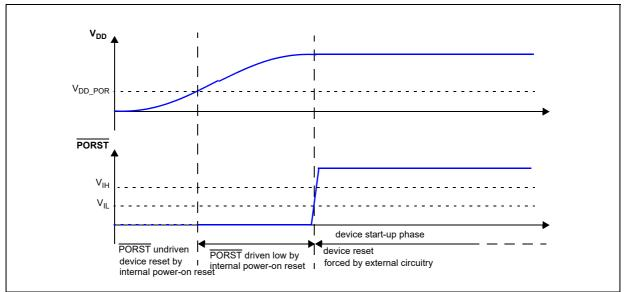
Figure 5. Startup reset requirements
