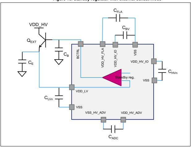
Figure 15. Standby regulator with external ballast mode
