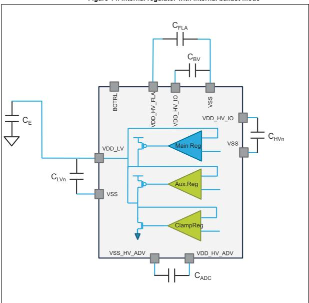
Figure 14. Internal regulator with internal ballast mode
