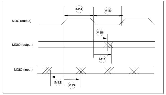
Figure 38. MII serial management channel timing diagram
