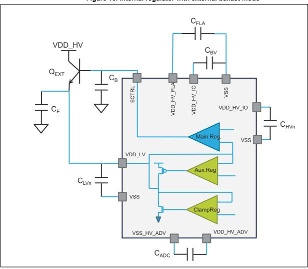
Figure 13. Internal regulator with external ballast mode
