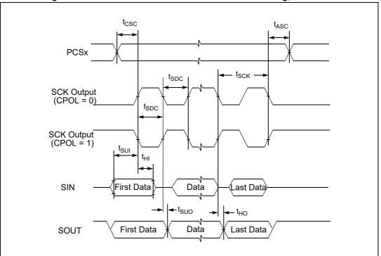
Figure 30. DSPI CMOS master mode — modified timing, CPHA = 0
