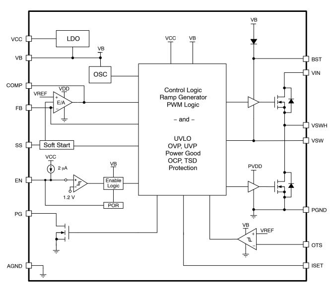
Figure 1. NCP3231A Block Diagram
