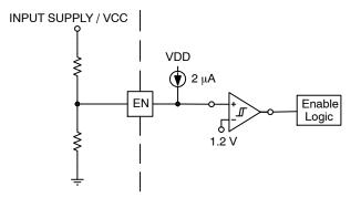
Figure 22. Enable Functional Block Diagram
