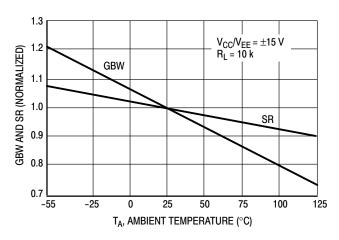
Figure 6. Normalized Gain Bandwidth Product and Slew Rate versus Temperature
