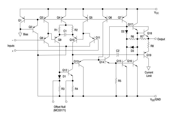
Figure 1. Representative Schematic Diagram (Each Amplifier)
