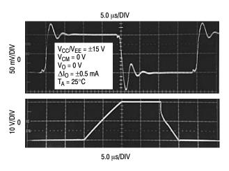
Figure 7. Small and Large Signal Transient Response
