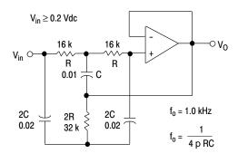
Figure 14. Active High-Q Notch Filter
