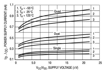
Figure 9. Supply Current versus Supply Voltage
