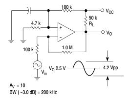
Figure 12. DC Coupled Inverting Amplifier
