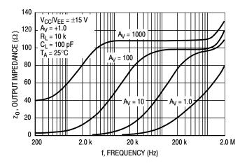
Figure 8. Output Impedance and Frequency
