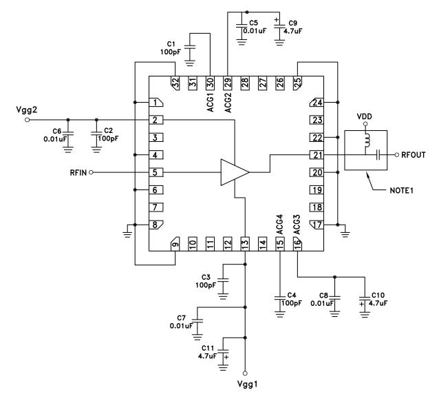
NOTE 1: Drain Bias (Vdd) must be applied through a broadband bias tee or external bias network.
