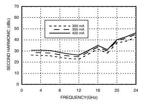
Vdd @ Pout = 18 dBm, Idd = 400 mA [1]  $70 \\ 60 \\ 50 \\ 40 \\ 40 \\ 20 \\ 10 \\ 0 \end{bmatrix}$
