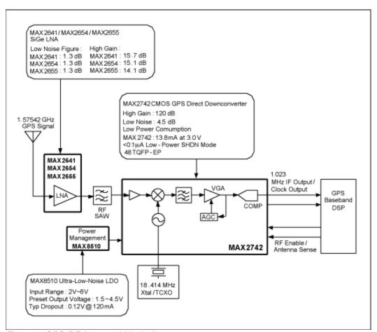
Figure 1. GPS RF front-end block diagram.
