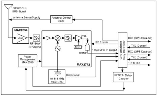
Figure 3. Complete GPS receiver solution block diagram.
