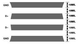
Figure 34. Arrangement of Signal Tracks
