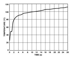
Figure 13. Response to Thermal Shock
