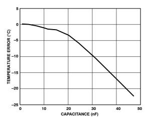
Figure 7. Temperature Error vs. Capacitance
