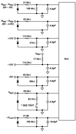
Figure 26. Voltage Measurement Inputs
