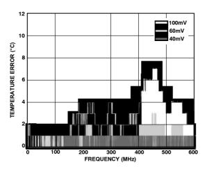
Figure 5. Temperature Error vs. Common-mode Noise Frequency
