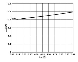
Figure 10. Supply Current vs. Supply Voltage
