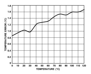
Figure 11. Local Sensor Temperature Error
