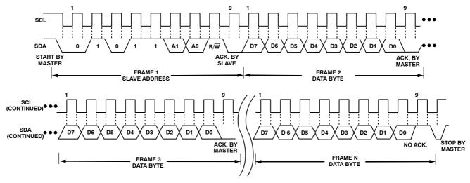
Figure 17. General SMBus Read Timing Diagram
