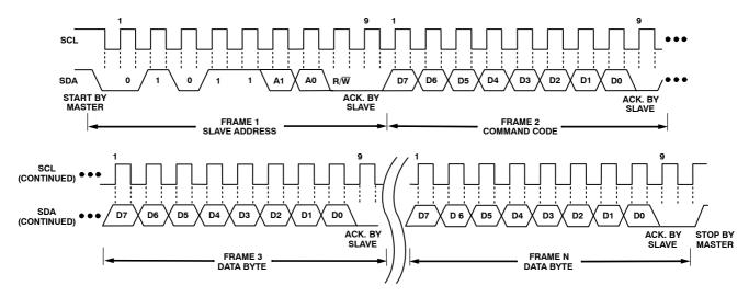
Figure 16. General SMBus Write Timing Diagram
