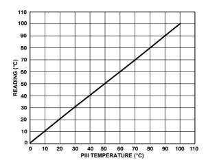
Figure 6. Pentium® III Temperature vs. ADM1026 Reading
