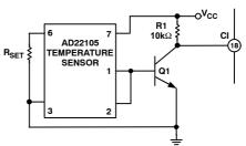
Figure 48. Using the CI Input with a Temperature Sensor
