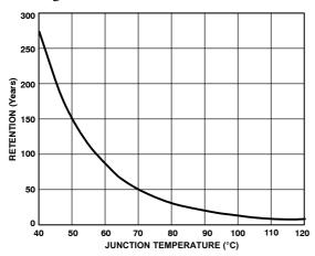
Figure 15. Typical EEPROM Memory Retention
