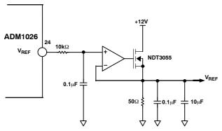
Figure 32. V<sub>REF</sub> Interface Circuit for V<sub>REF</sub> Loads > 2 mA
