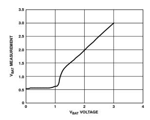
Figure 14. V<sub>BAT</sub> Measurement vs. Voltage
