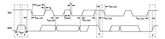
Figure 2. Serial Bus Timing Diagram
