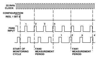
Figure 47. Fan Speed Measurement
