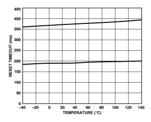
Figure 9. Powerup Reset Timeout vs. Temperature
