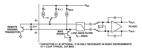
Figure 33. Signal Conditioning for Remote Diode Temperature Sensors
