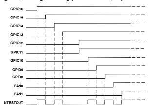
Figure 60. NAND Tree Test with Two Inputs Shorted
