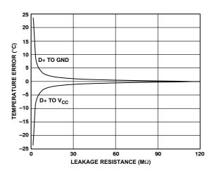
Figure 3. Temperature Error vs. PCB Track
