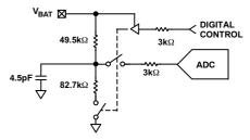
Figure 30. Equivalent V<sub>BAT</sub> Input Protection Circuit
