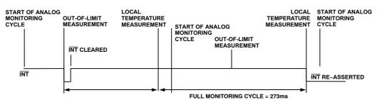
Figure 49. Delay After Clearing INT Before Reassertion
