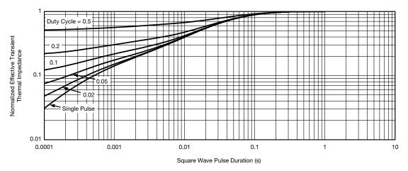
Normalized Thermal Transient Impedance, Junction-to-Foot
