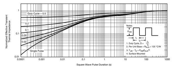
Normalized Thermal Transient Impedance, Junction-to-Ambient
