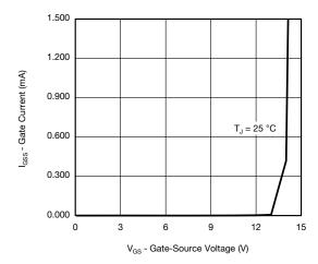
Gate Current vs. Gate-to-Source Voltage
