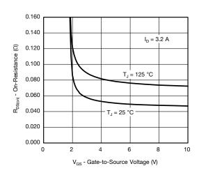
On-Resistance vs. Gate-to-Source Voltage
