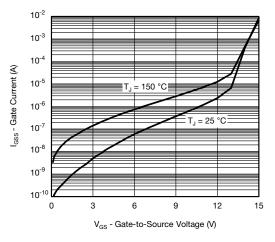
Gate Current vs. Gate-to-Source Voltage
